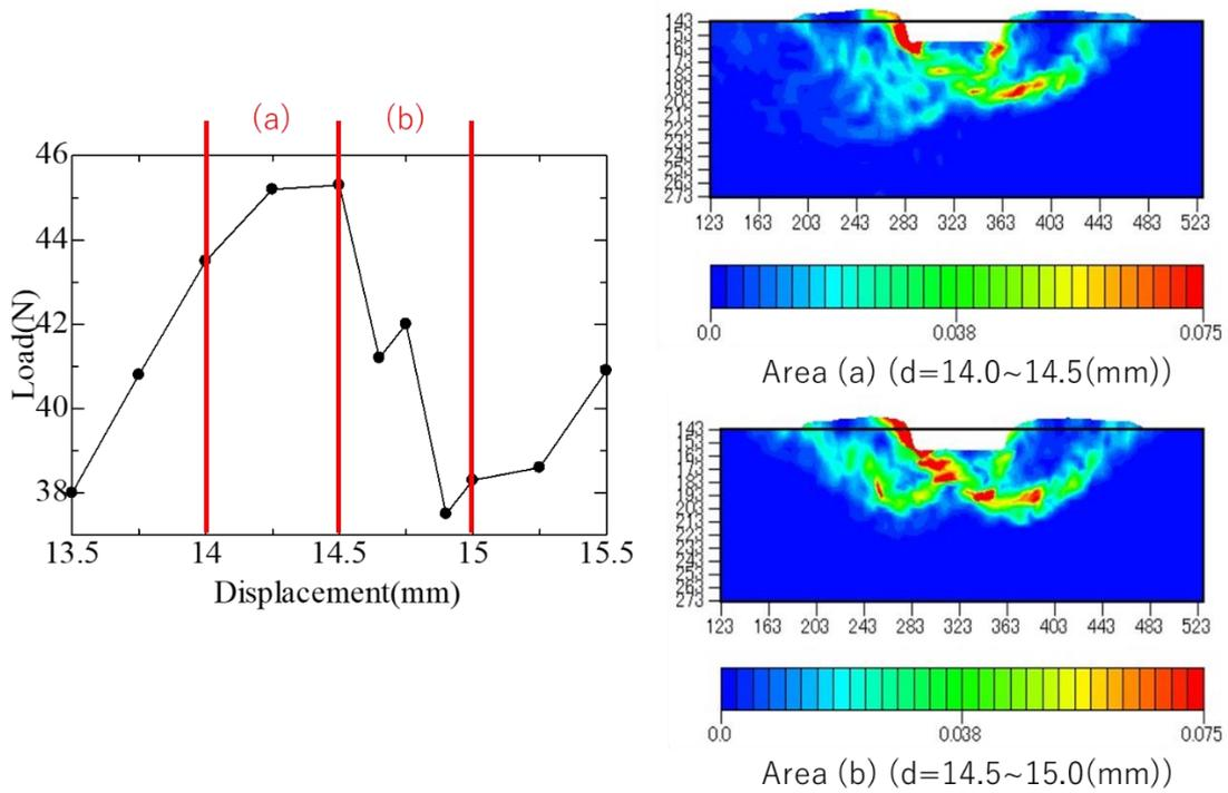
Figure 11: Example of comparison of PIV results and chart of loading versus displacement
