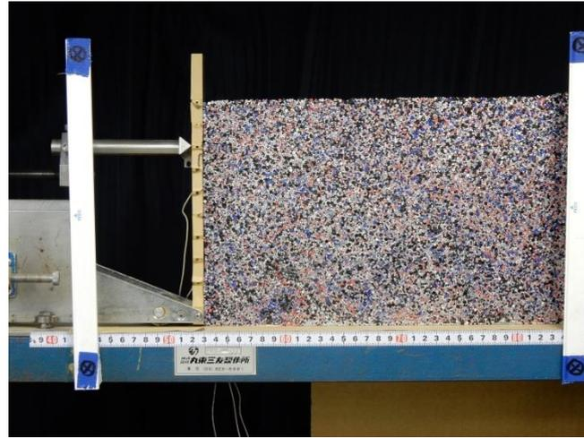
**Figure 3:** Arrangement of retaining wall test equipment
