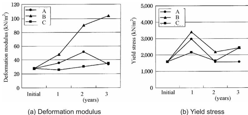
Figure 4. Variation of deformation modulus and Yield stress from LLT.
