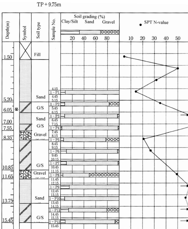
Figure 1. Soil profile, soil composition and SPT N-value of test field.
