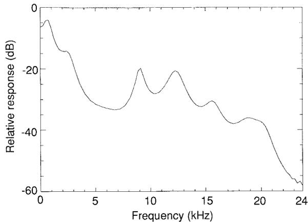
Fig. 4. Frequency response of transfer function with the estimated common AR coefficients.
