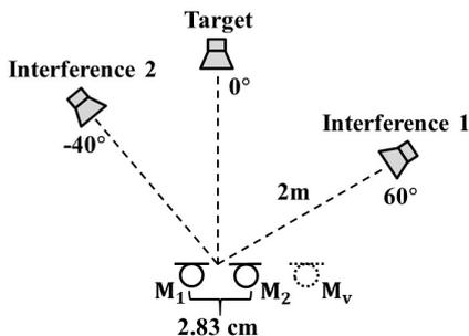
Fig. 3. Layout of sound sources and microphones in experiment.
