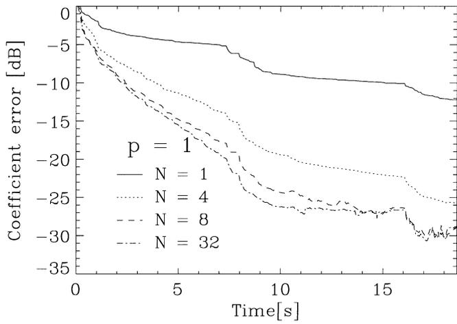
Fig. 9 Coefficient error convergence for speech input when  $p = 1$  NLMS algorithm.
