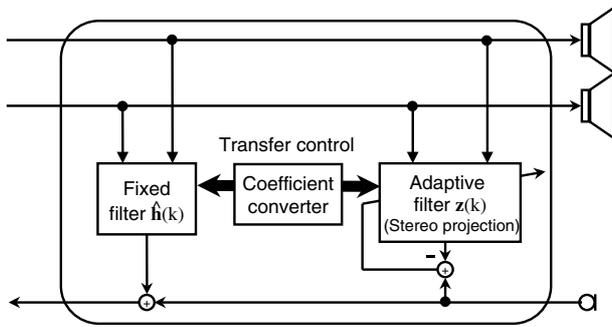
Fig. 12 Stereo duo-filter structure.
