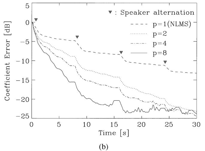
**Fig. 8** Convergence for speech input with stereo projection algorithm.
