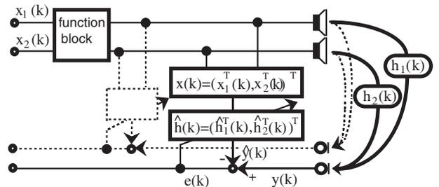
Fig. 5 Configuration of a stereo echo canceller with a function block.
