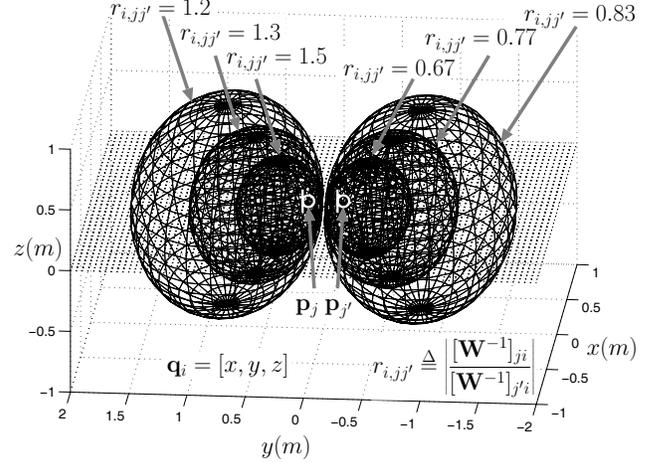
**Fig. 2.** Example of spheres determined by eq.(8) ( $\mathbf{p}_j = [0, 0.15, 0]$ ,  $\mathbf{p}_{j'} = [0, -0.15, 0]$ )
