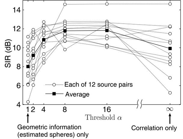
Fig. 4. Experimental results. SIRs are evaluated for 12 combinations of source signals with various values for threshold parameter  $\alpha$ .
