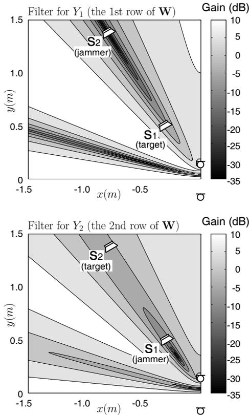
**Fig. 5.** Example of spatial gain patterns of separating filters ( $f = 1000$  Hz)
