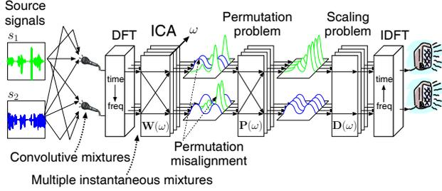
**Fig. 1.** Flow of frequency domain blind source separation
