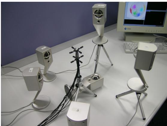
Figure 1: Prototype system (8 microphones and 6 loudspeakers)
