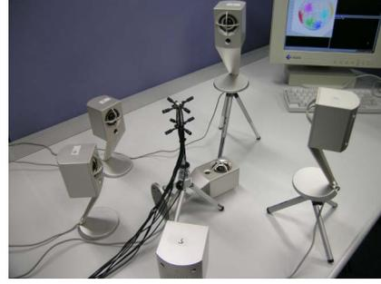
Fig. 5. Six 3-D located source signals and eight microphones located at the vertex of a 4 cm cube
