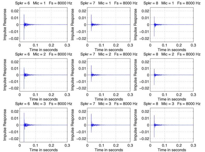
Fig. 4. Impulse responses measured from the uniform linear array,  $RT = 300$  ms condition.
