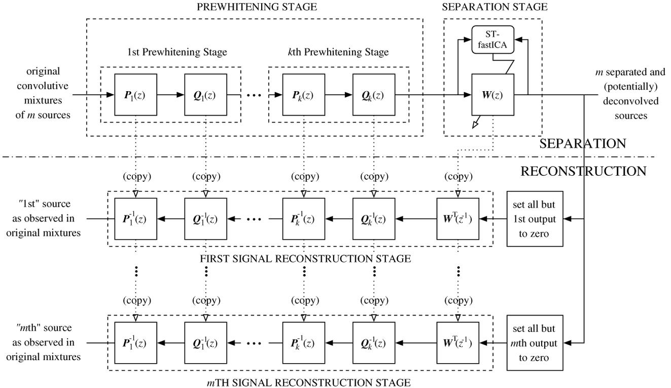
Fig. 2. Block diagram of the combined separation and signal reconstruction system.
