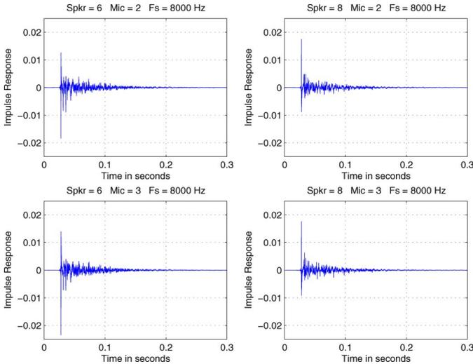
Fig. 5. Impulse responses measured from the uniform linear array,  $RT = 425$  ms condition.
