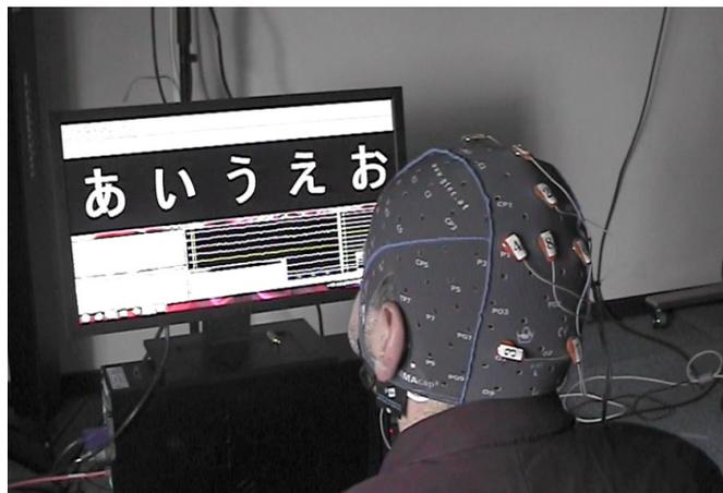
Fig. 1. Visual, auditory and audiovisual BCI speller test paradigm environment based on BCI2000 software [8]. The subject in the picture wears also EEG g.SAHARA electrodes connected to g.MOBllab+ amplifier by g.tec. In this paper we conduct the psychophysical and the preliminary EEG, in offline BCI setting, experiments to evaluate possible differences related to various stimulus perceptions.
