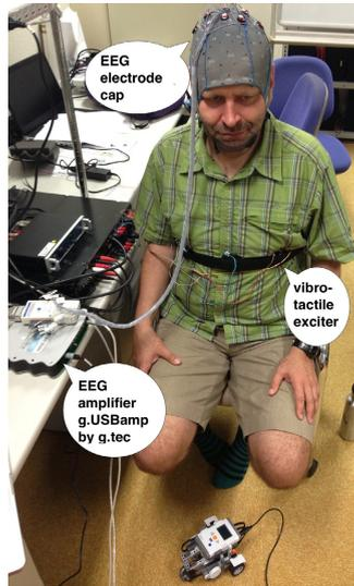
**Fig. 1.** Subject wearing EEG cap with 16 active electrodes attached to the g.USBamp amplifier. The five vibrotactile transducers are attached to an elastic belt on the subject chest. Small vehicle robot by LEGO MINDSTROMS, operated via tBCI application developed by the authors, is placed on the floor in front of the subject in the picture.
